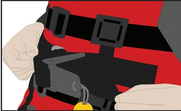
1. FOR IN WATER RESCUE OPERATIONS: thread the webbing through the plastic quick-release buckle only as shown. (see illustration in fig 6)
