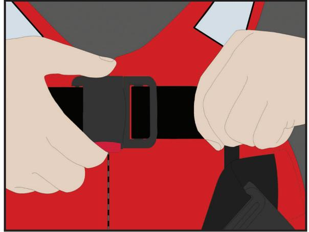
Tighten the top black webbing strap by holding the buckle with one hand and pulling the black webbing strap to the left with the other hand as shown. (see illustration in fig 4)
