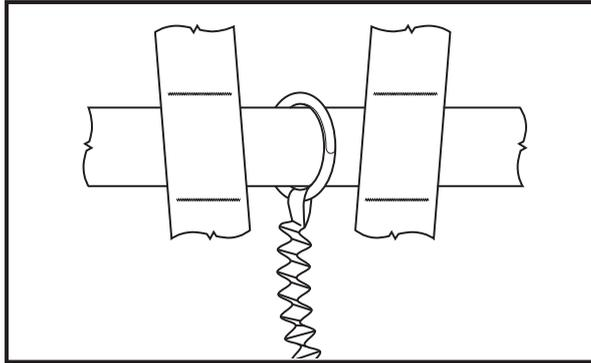
1. Open the fix lock buckle located on the front of the PFD and un-thread the webbing belt.
