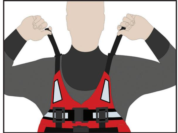
Finally take the two shoulder straps and pull forward simultaneously to ensure the correct adjustment.
