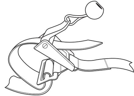
Close the buckle firmly checking that the webbing is not twisted during threading.
